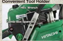
Keeps standard wrenches on the machine, preventing losses of them.
